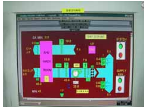
Honeywell central control system(例)
